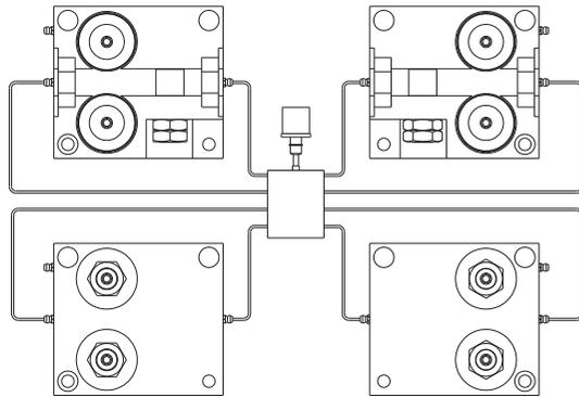
**Roller** Heavy duty lithium soap grease is filled inside the bearing before delivery. We recommend re-lubricate roller after each 1000Km working. In every roller housing, all of three rollers' lubricate holes are connected to roller housing's lubricate tube. So fill grease into the nozzle outside of the roller housing, each bearing will be re-lubricated. According to grease's properties, roller can be used between -30°C and 120°C working conditions.
