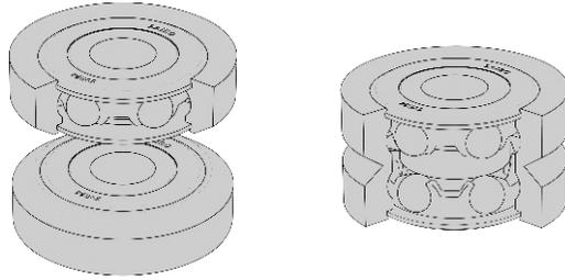
□ Twin type bearing      ■ Double row type bearing
