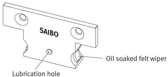
Plastic lubrication cover contains oil soaked felt wipers which can be re-lubricated via lubrication hole. This lubrication cover is optional, not included in standard carriage.
