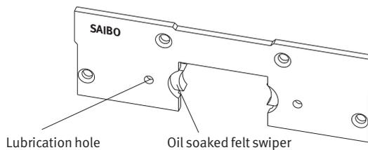
Plastic lubrication cover contains oil soaked felt wipers which can be re-lubricated via lubrication holes.
